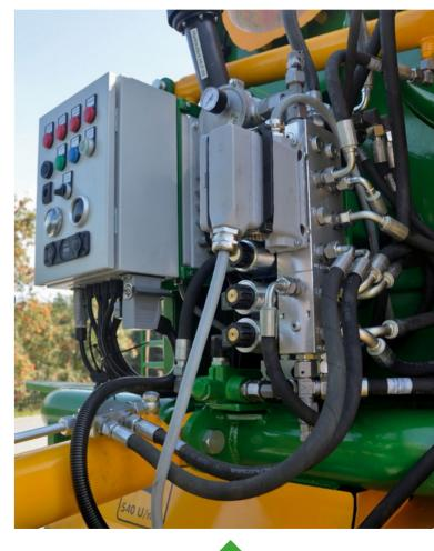
■ control block with electromagnetic ventils
