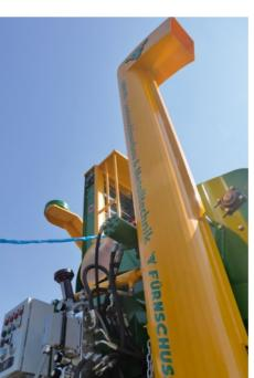
■ hydraulically outward-swinging auger tube with tailing elevator (no overhead hydraulic system)
